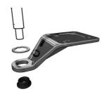
*Note:* The washers help to prevent the mirror mount from moving or from being damaged. Select the diameter of the washers according to the diameter of the bolt hole.
